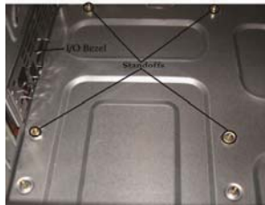
Fig. 2.1(p) : Fixing standoffs on the cabinet
