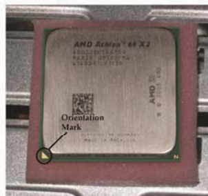
Fig. 2.1(i) : Orientation mark on a processor
