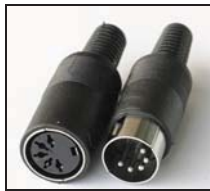
Fig. 1.9(b) : Female and male 5-pin DIN connectors
