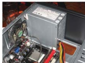
Fig. 2.1(g) : Installing the power supply unit
