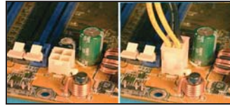
Fig. 1.8(j) : Connecting a P4 connector to the motherboard
