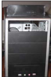
Fig. 2.1(r) : Cabinet with blanking panel removed
