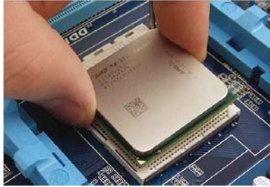
Fig. 2.1(j) : Inserting the processor into the socket
